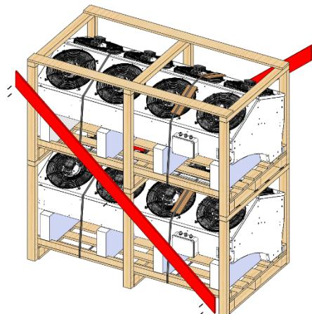
After the upper pallet is removed, disassemble the braces. The pallets are joined by screws that need to be unscrewed to remove the pallet.
