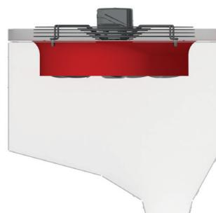
All AXI units are equipped with integrated fan diffuser in order to reduce the turbulent air flow inside the unit and thus increase the total air volume. This feature also reduces the noise generated by the fans. Thanks to the integrated fan diffuser the unit is fully compliant with ERP 2015 regulation.
